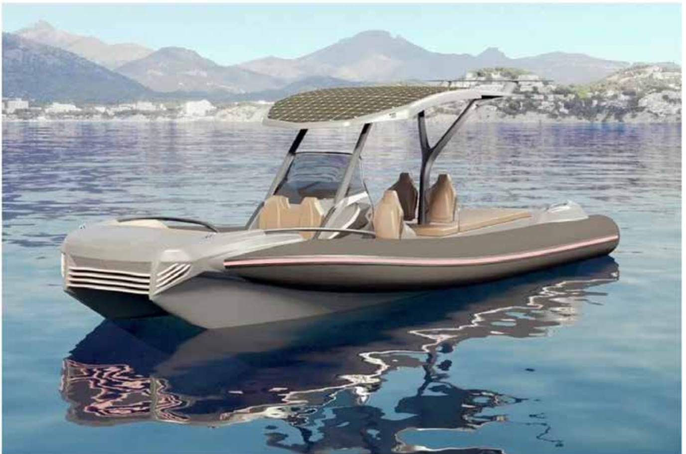
The Speed 28 is a carbon-fibre, twin-hulled RIB
