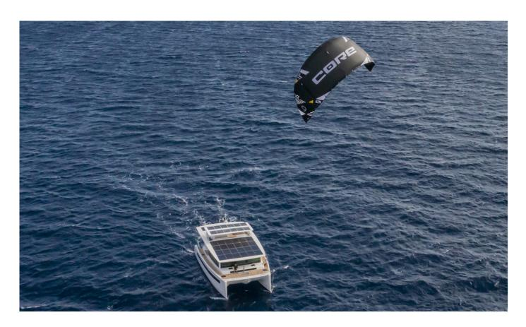
Electric yacht manufacturer Silent-Yachts has become the first boat builder to date to design and build boats for the use of a kite sail system with the unveiling of the SILENT 60 solar powered catamaran.
