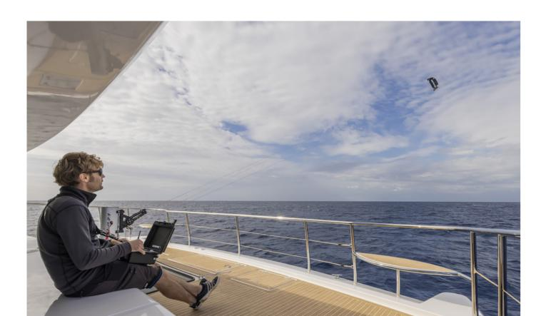
According to the brand, "after inflating the kite, it is released overboard to drift away on the surface of the water", while "pulling on the lines launches it into the air and once it reaches the optimal flight height, it begins to trace a figure 8 in the sky and generates power to pull the yacht".
