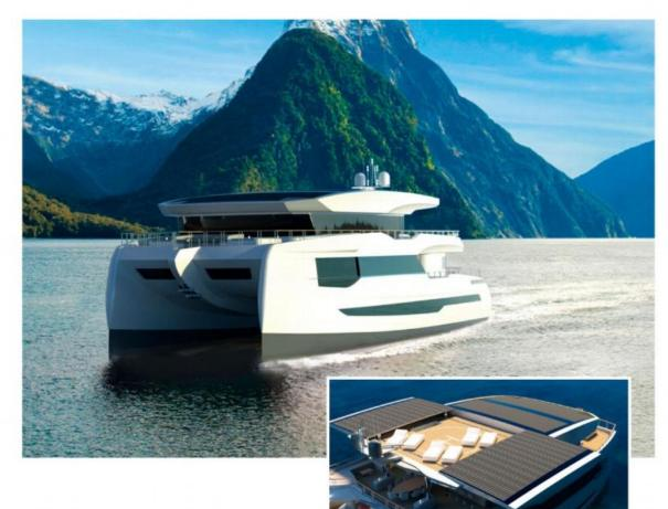
RIGHT: The supersized supercat features 40kWp of photovoltaic panelling
