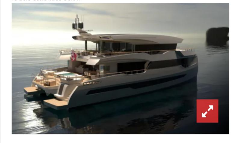
All that energy is then used to power two 340 kW electric motors. Even though this beast will weigh around 440 GT, it's still able to hit speeds upwards of 16 knots (18.4 mph), depending on the load. Technically, because it's solar-powered, Silent Yachts likes to boast that the 100 features an "infinite" range, as long as all systems function properly.
