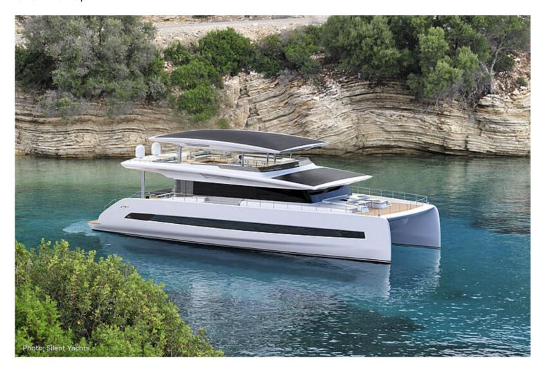
In addition to this restructuring, the shipbuilder will offer its first hybrid yacht, which will be built in partnership with VisionF Yachts. The Silent VisionF 82 will be a 25-metre catamaran equipped with solar panels and a battery pack that will provide the power for all household and comfort appliances onboard.
