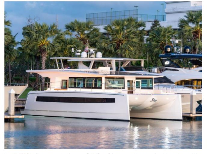
The SILENT 60 solar-powered catamaran is designed to go anywhere as a true bluewater cruising yacht. The first "Front Exit" version (four cabins) is equipped with twin electric motors of 250kW each, a Lithium-ion battery bank with a capacity of 225 kWh and a 150kW diesel generator. The yacht can cruise efficiently with zero emissions solely on solar power for up to 100 nautical miles a day.
