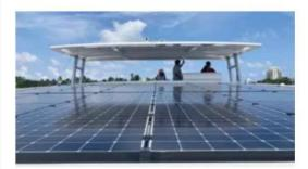
There are 42 panels on the roof and foredeck of the Silent 60, with a total electricity generation rating of 17kWp: kiloWatts peak, meaning 17 kiloWatts per hour can be generated under ideal conditions.
