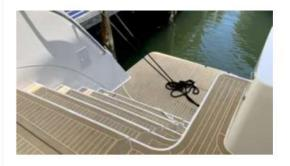
Stairways on either side lead down to swimming platforms and between them is the hydraulic platform/lift that can carry a 4 metre (13 ft) tender/dinghy or jetski (preferably electric). The draft of the 60 is under 1 metre (39") so it can access even the shallowest swimming areas and bays.
