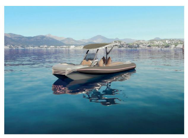
The boat is equipped with lithium-ion batteries (LiFePO4) storing around 100 kWh of energy.
