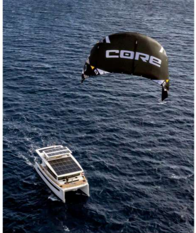
The sailing background of Silent-Yachts founders Michael and Heike Köhler (left) is evident in an optional kite that can add 3 knots of propulsion to the Silent 60.
