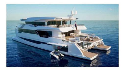
The new Silent 120 is scheduled to be launched in 2024. It's 120 feet long with a 45' 4" beam and it displaces 490 gross tons. It uses a series of 40-kWp solar panels to charge an 800-kWh lithium-ion battery bank. That, turn, powers two 340-kW electric motors, producing a top speed of 16 knots. The cat's most efficient speed is 8 knots.
