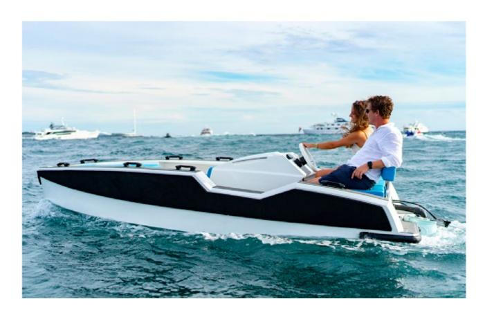
Its carbon fiber lay-up ensures that the hull of the sporty-looking tender weighs no more than 90kg. That means it is lighter to lift out using the hydraulic bathing platform of a Silent 60, easier for the mother ship to carry and crucially, far more efficient to propel through the water.
