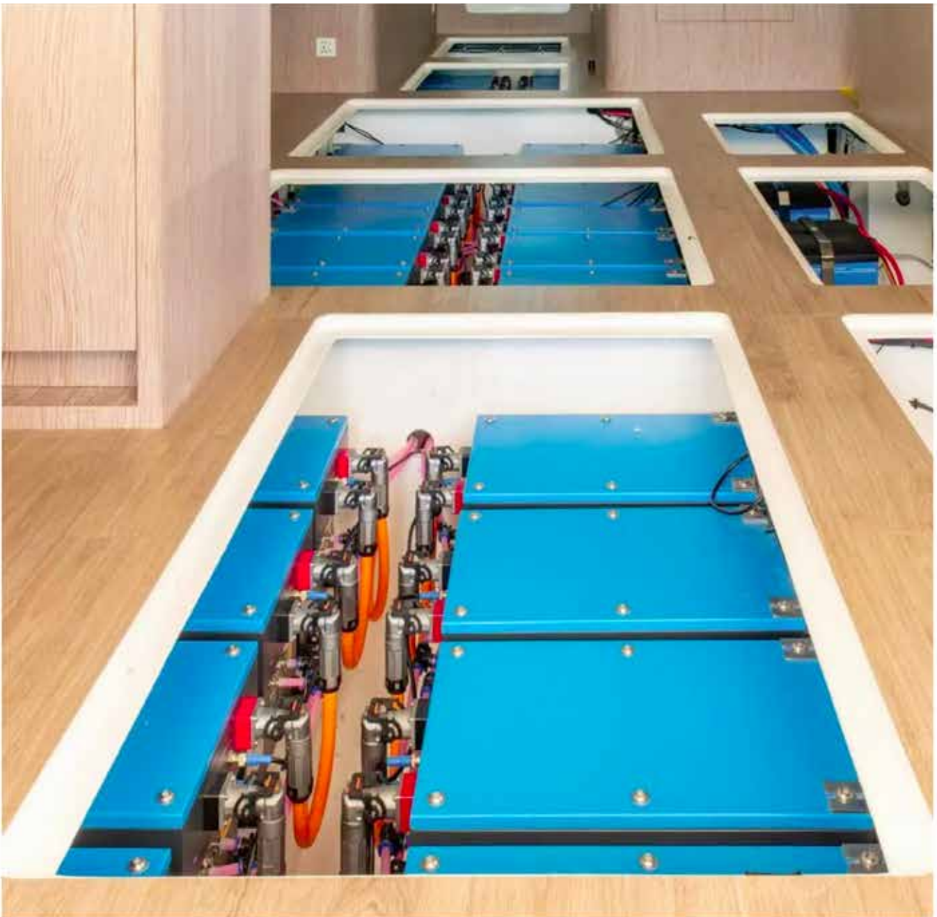
Silent 62 new drivetrain electric batteries
