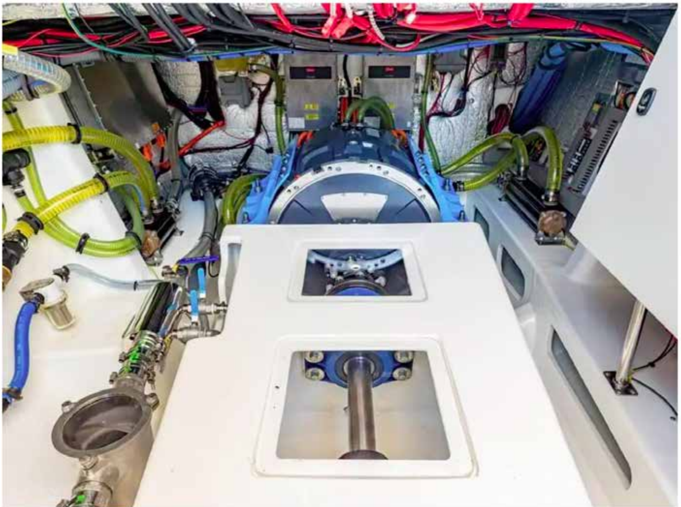
Silent 62 new drivetrain electric motors
