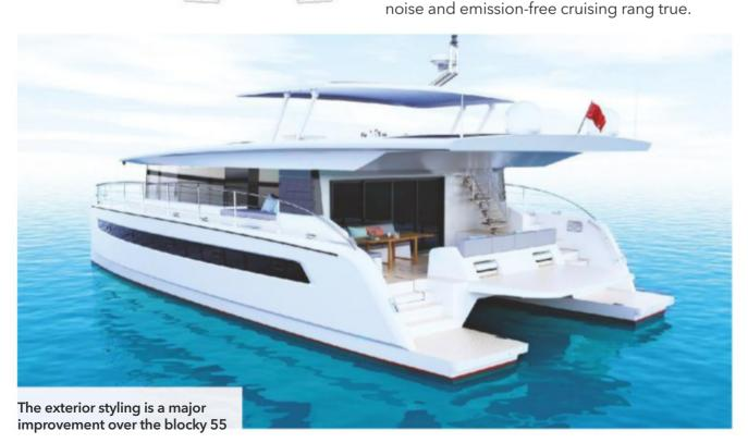
Enter the 60, with a redesigned hull that has a longer waterline and reverse bow to improve efficiency, and styling by Albert Nazarov that apes the flagship 80. The 55's awkward looks have been replaced by a design that is far kinder on the eye and makes room for even more living space plus a boost in solar power acreage on the roof from 30 to 42 panels.
