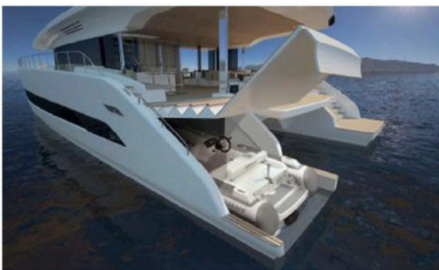
The absence of an engine room allows for a huge garage on the Silent 80 (left); the Silent 60 (right) is being built in Thailand by Bakri Cono
