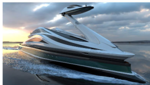
Avanguardia's 'nose' will lower to sea level and release a 16-metre tender. Image credit: Lazzarini design studio
