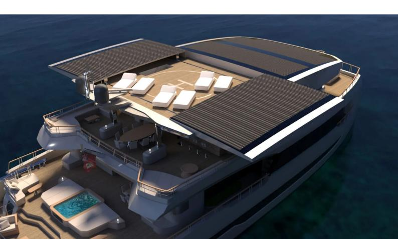
Spead across four decks, the yacht is fitted with a solar-electric drive train providing a cruising speed of 10 knots and a top speed of 14-16 knots.
