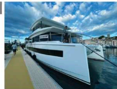
The bows are high and very tapered. This allows the catamaran to be more efficient in choppy water and to maintain good bridge-deck clearance.
